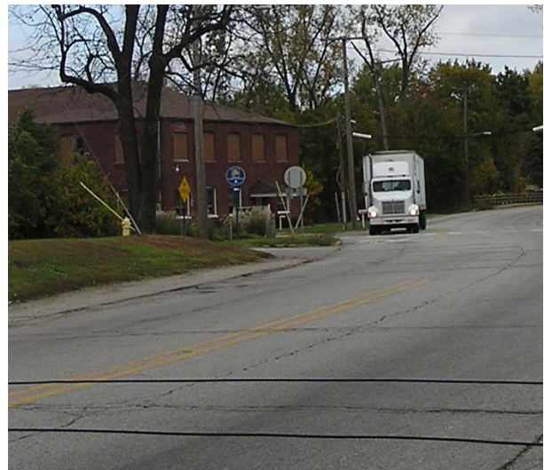
Figure 1. Truck preparing to cross traffic count tubes (foreground) on State Road 4 in Goshen, IN.
